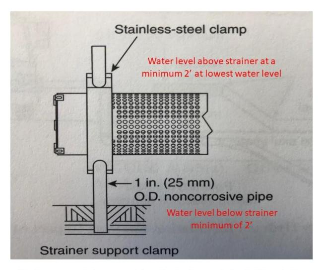
Strainer support clamp must be attached to a substantial foundation block, approved by Wilton Fire.
