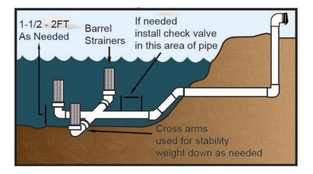
Cross arms must be supported by a substantial foundation block or blocks, approved by Wilton Fire.
